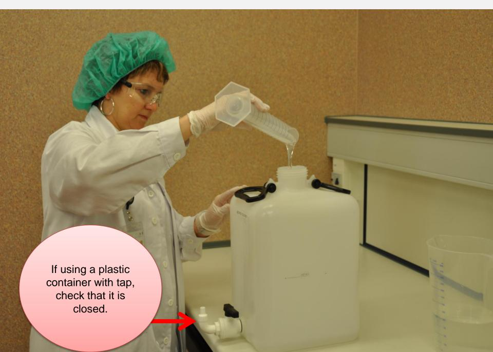
Pour the measured quantity of hydrogen peroxide 3% into the final recipient
