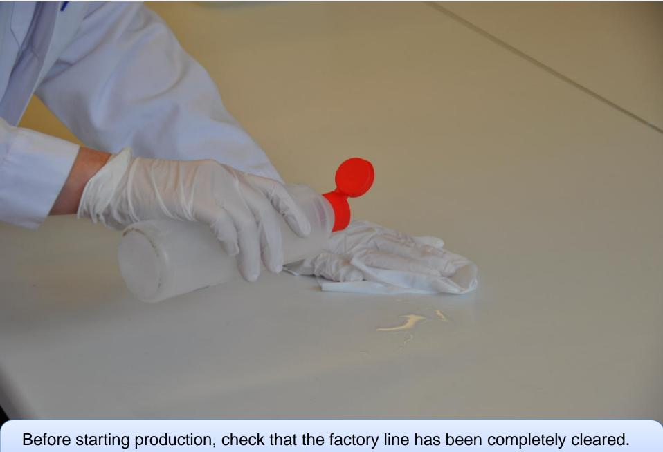
Before starting production, check that the factory line has been completely cleared. That is to say, ensure that the working area is free of any unnecessary raw ingredients and materials, and that it has been cleaned with alcohol.
