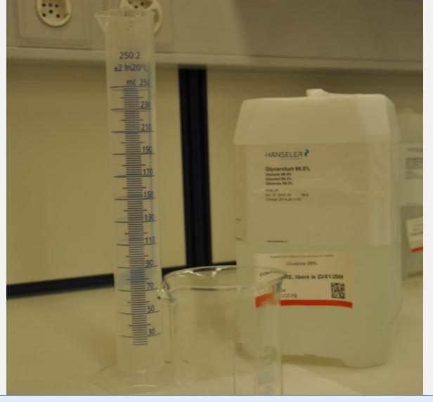
Set out on the workplace the amounts of raw ingredients required for production. Check that the names and quantities are consistent with the manufacturing documents and check their validity (expiration dates in relation to the period of use of the finished product).
