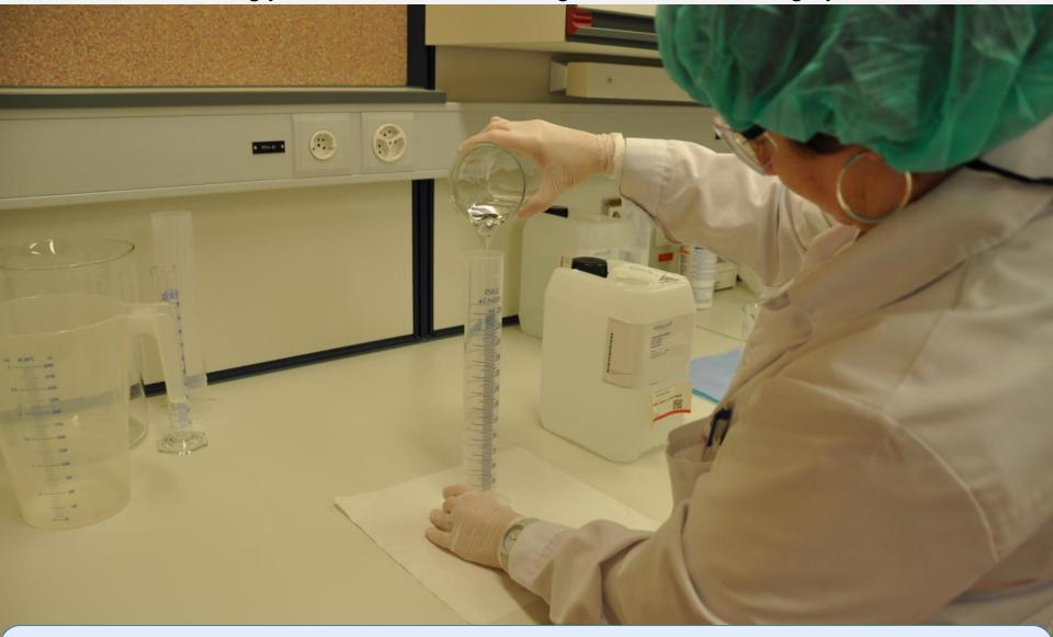
Try to avoid letting the viscous glycerol run down the side of the cylinder. Wait until all the bubbles formed have risen to the surface in order to be able to note the exact level of glycerol in the measuring cylinder.
