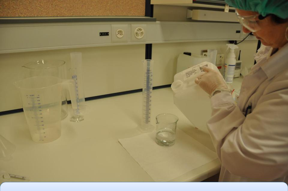
To facilitate measurement in the measuring cylinder, use a funnel or transfer into a beaker beforehand.
