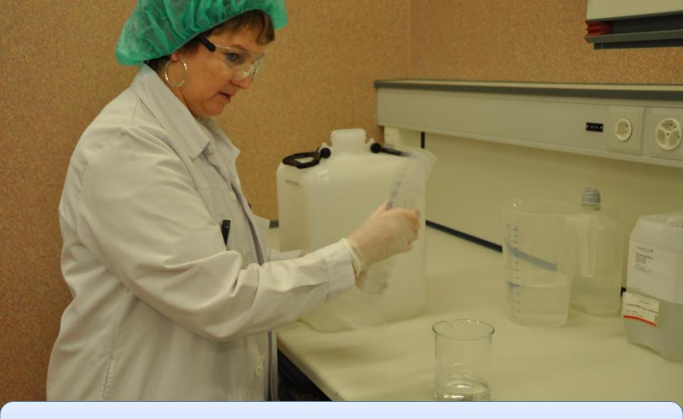
Then rinse the cylinder that was used for the glycerol with some ethanol (using ethanol from the amount already measured), until all glycerol residues have been removed.
