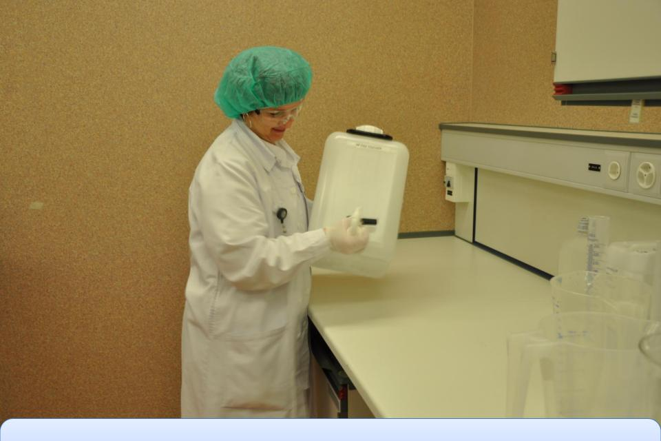
Close the container with the screw cap as quickly as possible to prevent any evaporation and then gently mix by shaking the recipient for 5 minutes.
