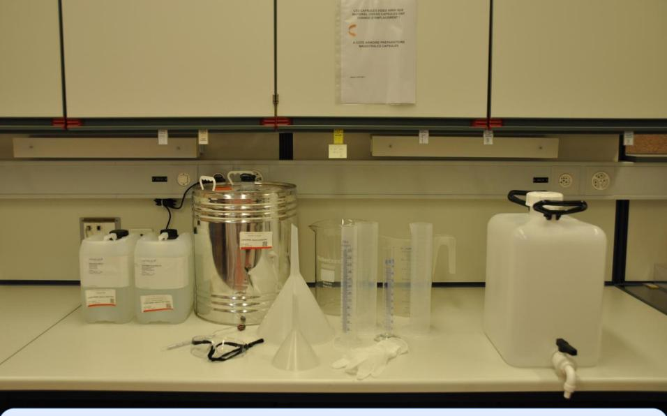
Set out all the equipment needed for production and check that it is clean. If necessary, calibrate the final container for the volume of 10 liters by drawing a mark on it (engraving this mark is recommended to prevent its erasal by alcohol or other substances).
